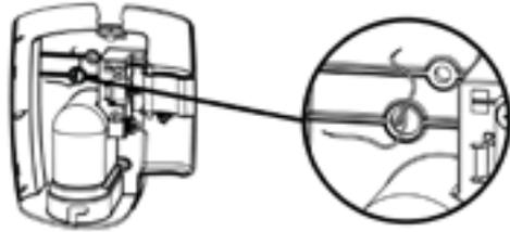
6. Then, fix the console onto its mounting plate with the three short screws (#10 3/4").
