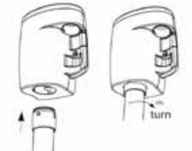
12. Insert the nozzle into the console. The installation of the WallyFlex is now completed.
