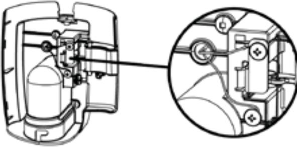
8. Close the front panel of the console, ensuring the tabs on the door and console are properly aligned, and fix screw #2.
