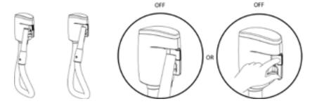
**Note:** When in use, for increased safety, the central vacuum unit can be stopped at any time, simply by pressing the switch on the WallyFlex console.
