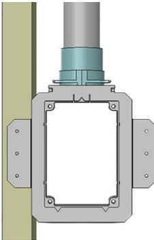
Install the pipe into the fitting.
