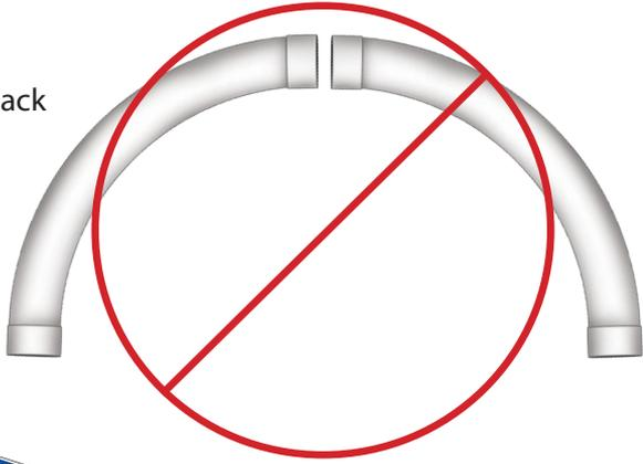
It is important to design the pipe runs so the hose is stored on one plane.
