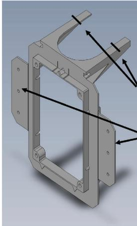
To allow the frame to fit through the valve hole in the sheetrock, cut approximately 3/4" (1.9 cm) off the forks.
