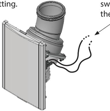
Using wire nuts, connect the two leads from the switch that is mounted on the outside of the valve to the low voltage wire.
