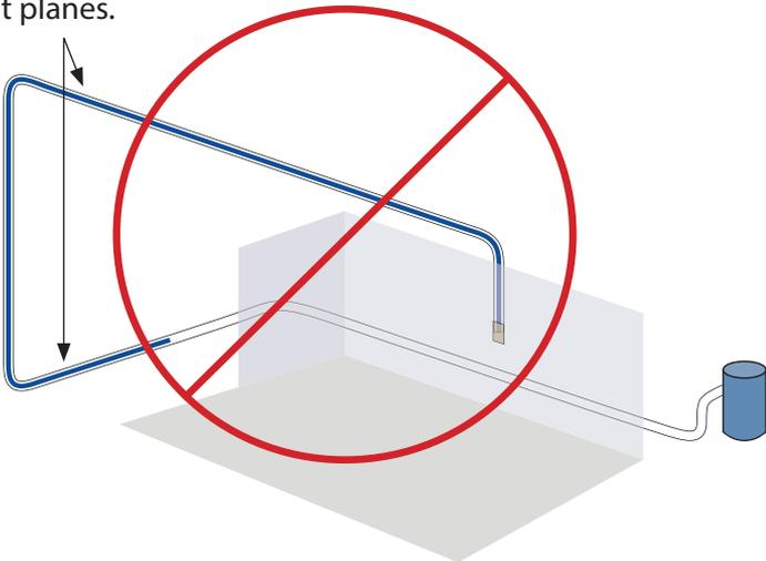
When using the Rapid Flex hose, we recommend installation of a reducer in the pipe run, before the first standard fitting. This prevents the possibility of the hose getting stuck in a tight fitting, if it stretches when retracted. See diagram below for positioning.
